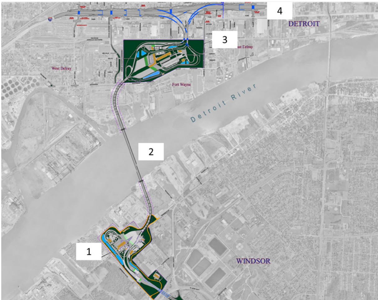
Figure 1: Components of the Gordie Howe International Bridge
